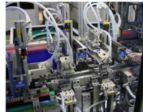
Automatic assembly of terminal block assemblies
