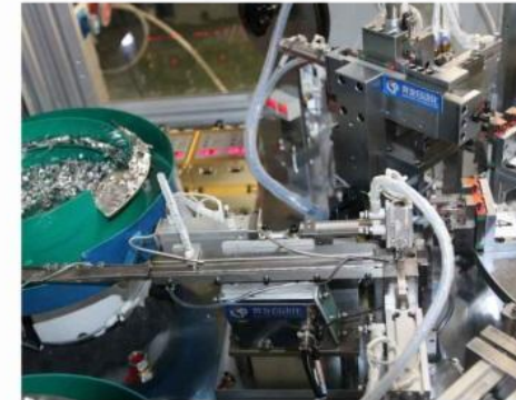
MCB miniature circuit breaker magnetic assembly / coil assembly automatic welding equipment
