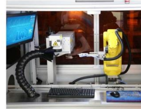
MCB miniature circuit breaker robot + automatic plastic housing loading equipment
