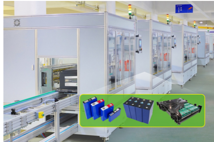
Lithium battery module pack automatic assembly and testing production line
