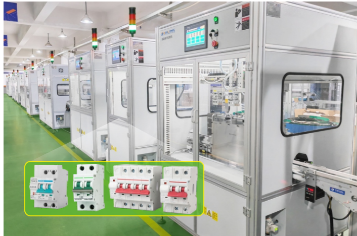
Photovoltaic reclosing DC circuit breaker automatic assembly and testing production line
