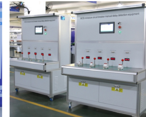
MCB manual time-delay testing equipment
