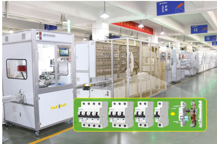
MCB miniature circuit breaker automatic assembly and testing production line
