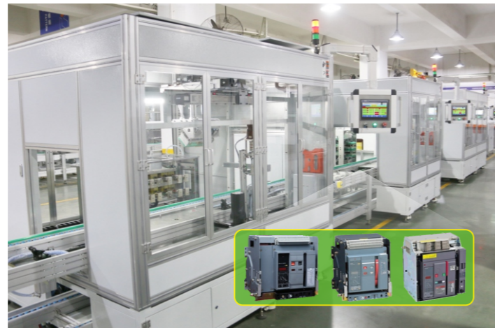
ACB Frame Circuit Breaker Automated Assembly and Testing Production Line
