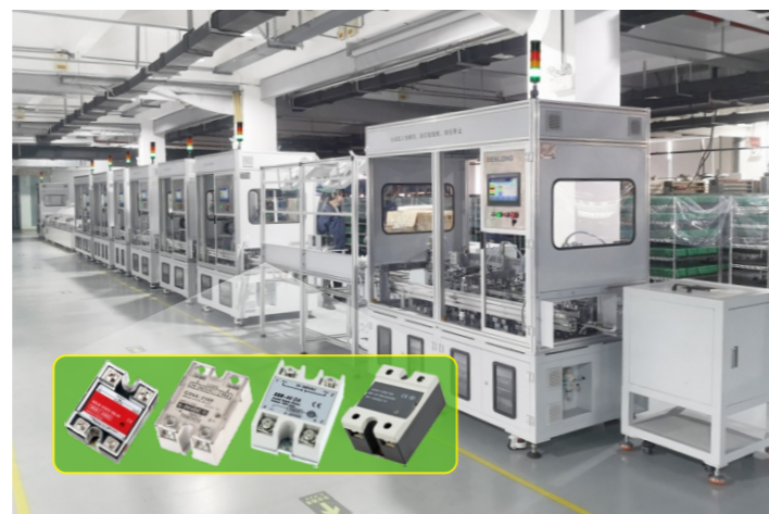
SSR State Relay Automated Assembly and Testing Production Line
