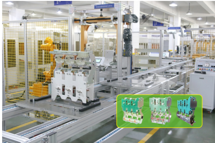
Automatic assembly and testing production line for vacuum circuit breaker of inflatable cabinet
