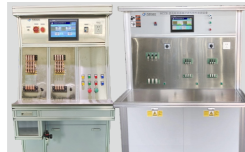
MCCB Molded Case Circuit Breaker Manual Instantaneous Testing Equipment
