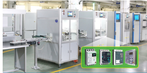
Automatic assembly and testing flexible production line for measuring switches
