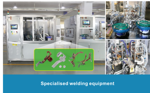
Photovoltaic reclosing/DC circuit breaker automatic assembly and testing flexible production line
