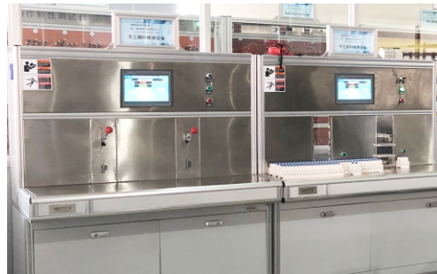
MCB miniature circuit breaker manual instantaneous testing equipment
