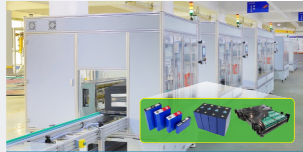
Lithium battery automatic assembly and testing flexible production line
