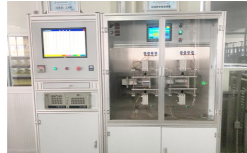
MCB miniature circuit breaker mechanical life testing equipment
