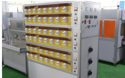
RCBO Leakage Circuit Breaker Aging Test Equipment
