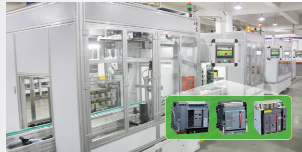
ACB frame circuit breaker automatic assembly and testing flexible production line
