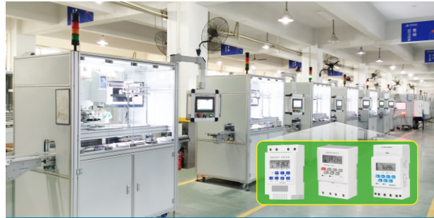
Automatic assembly and testing flexible production line for time control switches
