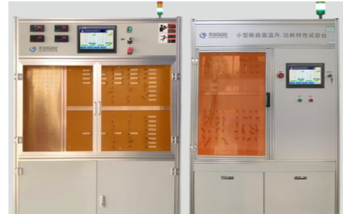
MCB miniature circuit breaker temperature rise, power consumption testing equipment
