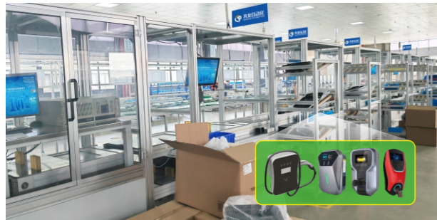
Flexible production line for automated assembly and testing of AC charging piles
