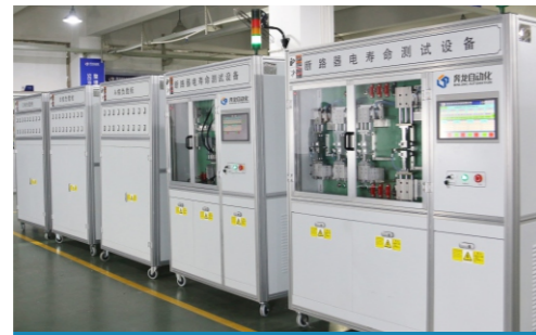
MCCB Molded Case Circuit Breaker Electrical Life Testing Equipment
