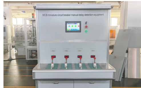
MCB miniature circuit breaker manual delay testing equipment
