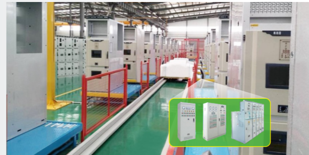
Intelligent control cabinet automatic assembly and testing flexible production line
