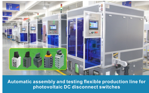
Photovoltaic reclosing/DC circuit breaker automatic assembly and testing flexible production line
