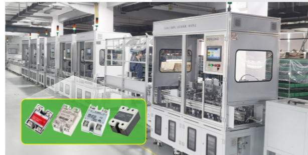
Automated assembly and testing production line for solid state relays
