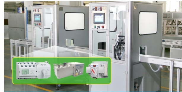
Double power automatic transfer switch automatic assembly and testing flexible production line
