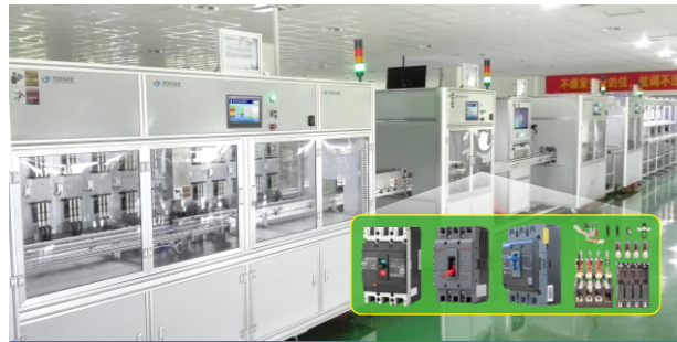
MCCB flexible production line for automated assembly and testing of moulded case circuit breakers
