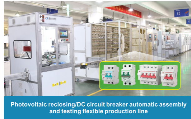
Automatic assembly and testing flexible production line for photovoltaic DC disconnect switches
