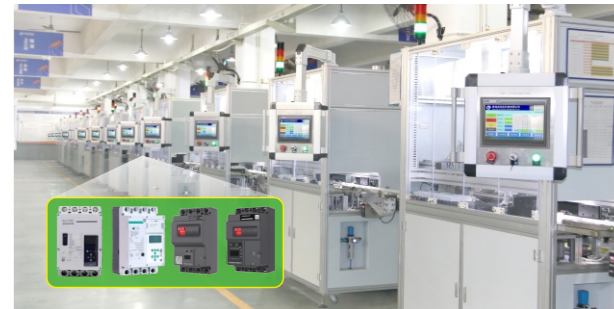
Low-voltage magnetron switch automated assembly and testing flexible production line
