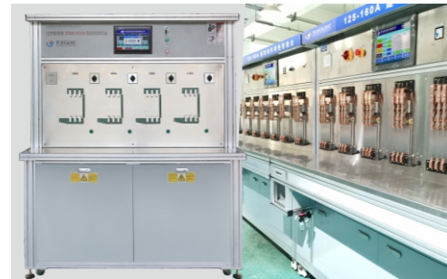
MCCB Molded Case Circuit Breaker Manual Delay Testing Equipment
