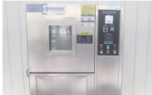
MCB miniature circuit breaker high and low temperature testing equipment
