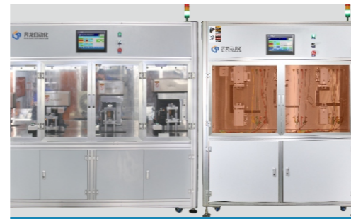
MCCB Molded Case Circuit Breaker Mechanical Life Testing Equipment
