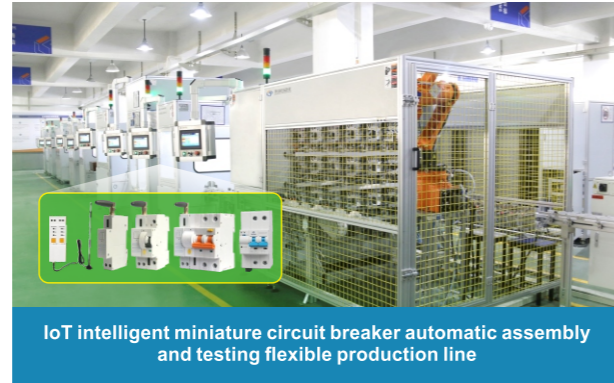
MCB miniature circuit breaker automatic assembly and testing flexible production line
