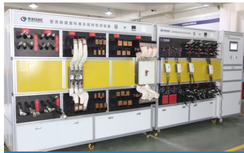
MCCB molded case circuit breaker standard long delay testing equipment
