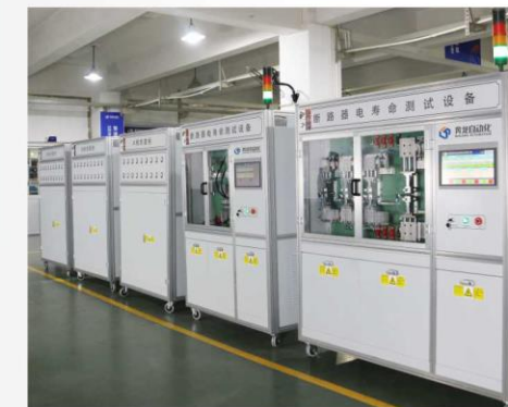
MCB/MCCB微型断路器电寿命检测设备 MCB/MCCB Electrical Life Testing Equipment
