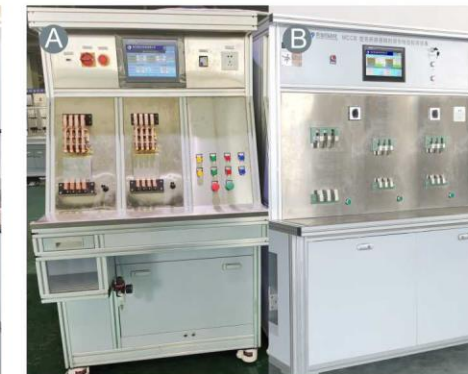
MCCB塑壳断路器手工瞬时检测设备 MCCB manual transient detection equipment
