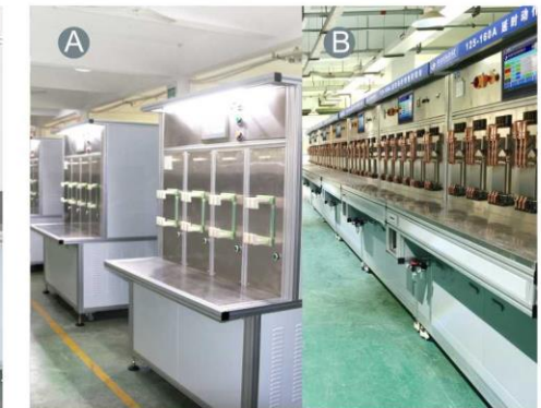
MCCB塑壳断路器手工延时检测设备 MCCB manual delay detection equipment
