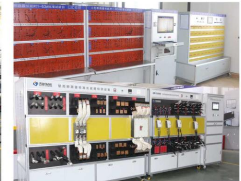
MCB/MCCB标准长时延测试设备 MCB / MCCB standard long delay testing equipment
