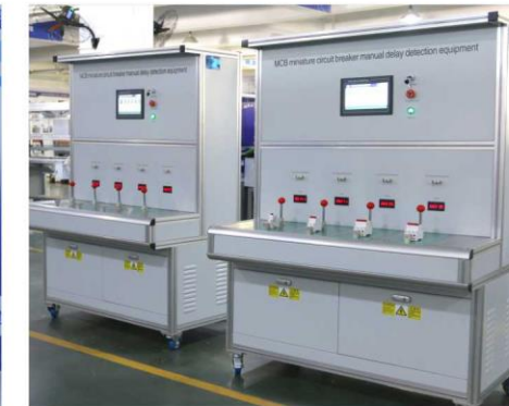
MCB微型断路器手工延时检测设备 MCB manual time-delay testing equipment
