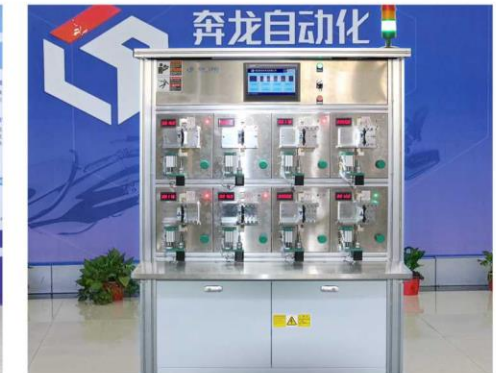
MCB微型断路器半自动延时检测设备 MCB semi-automatic time-delay testing equipment
