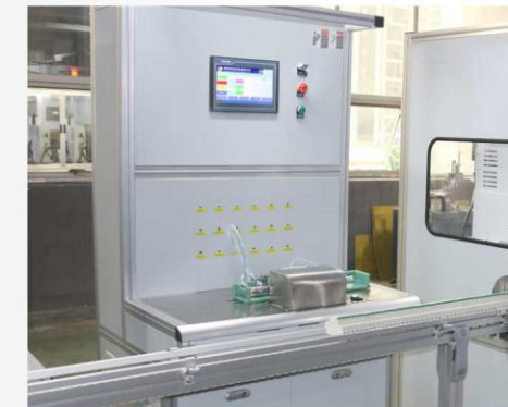
MCB微型断路器半自动瞬时检测设备 MCB semi-automatic instantaneous testing equipment
