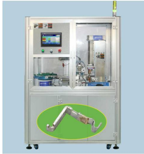
接线板组件自动焊接设备 Automatic welding equipment for terminal block assembly
