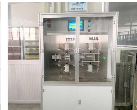
MCB/MCCB微型断路器机械寿命检测设备 MCB/MCCB Mechanical Life Testing Equipment
