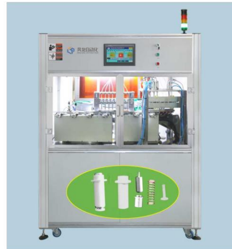
铁芯组件自动装配设备 Automatic assembly equipment for iron core assembly
