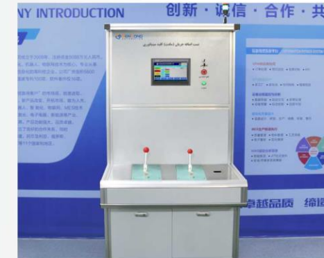
MCB微型断路器手工瞬时检测设备 MCB Manual Instantaneous Testing Equipment
