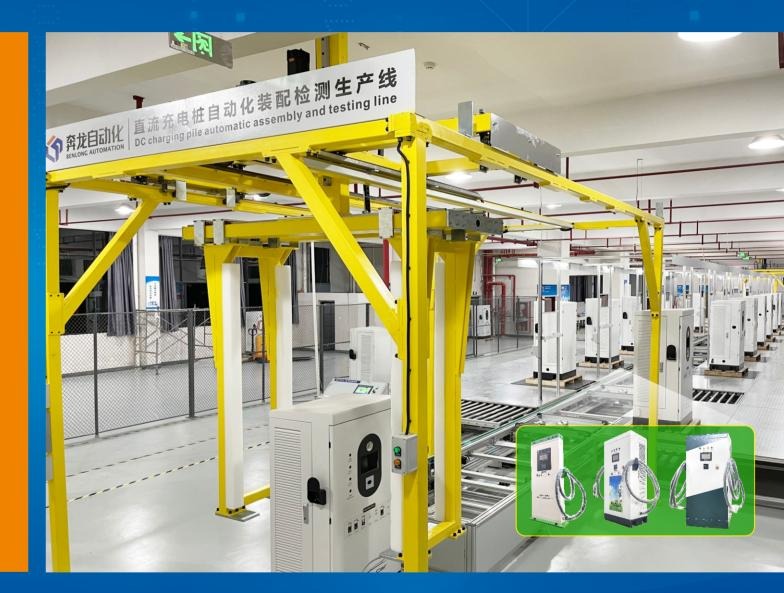
DC CHARGING PILE AUTOMATIC ASSEMBLY AND TESTING FLEXIBLE PRODUCTION LINE
