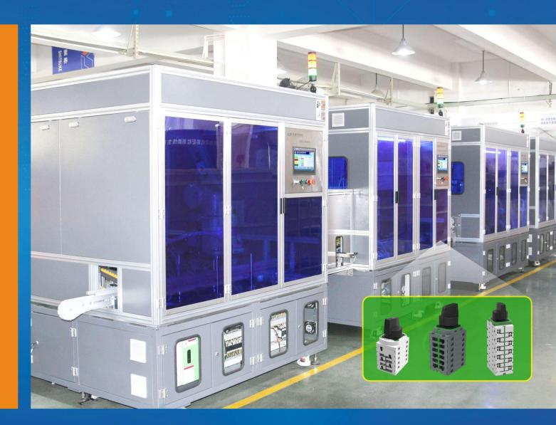
**AUTOMATIC ASSEMBLY AND TESTING FLEXIBLE PRODUCTION** LINE FOR PHOTOVOLTAIC DC DISCONNECT SWITCHES
