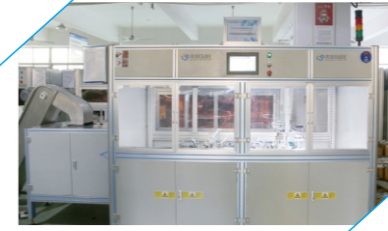
MCB微型断路器视觉检测设备 MCB miniature circuit breaker visual inspection equipment
