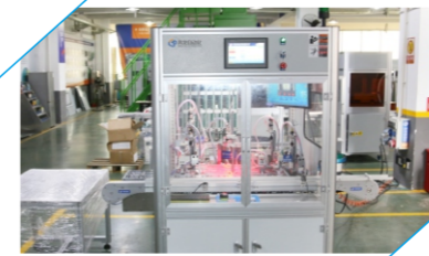
MCB微型断路器自动穿铆钉检测设备 MCB miniature circuit breaker automatic riveting inspection equipment
