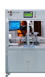
MCCB塑壳断路器自动激光打标设备 MCCB plastic case circuit breaker automatic laser marking equipment
