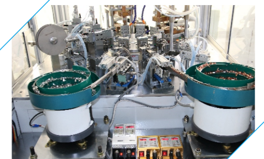
MCB微型断路器磁组件或线圈组件自动成型、检测、冲压、焊接一体化设备 MCB miniature circuit breaker wire, temperature sensing piece, terminal block automatic welding equipment
