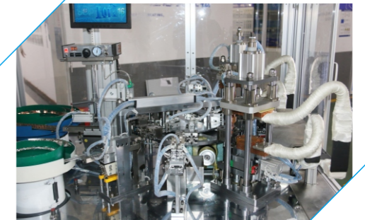
MCB微型断路器磁轭、银点、引弧角自动焊接设备 MCB miniature circuit breaker magnetic assembly or coil assembly automatic forming, testing, stamping, welding integrated equipment
