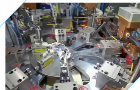
MCB微型断路器导线、温度感应片、接线板自动焊接设备 MCB miniature circuit breaker magnetic assembly or coil assembly automatic welding equipment
