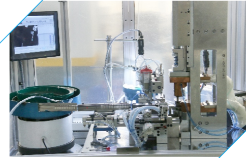
MCB微型断路器银点、静触头自动焊接设备 MCB miniature circuit breaker double gold, dynamic contact, braided wire automatic welding equipment
